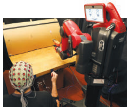
Robots that are sensitive to brain and muscle signals from a humans, like this drill-wielding bot with a human controller, could make for better assistants in factories or homes.
