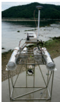
An experimental robot for hunting down and slicing up jellyfish can float in small jelly-terminator packs.
