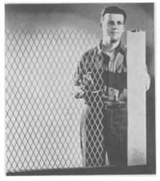
openings, but is made from solid sheets in a huge press with a serrated knife blade, as illustrated in the photograph. After cutting it is stretched to a width of some 10 times that of the original sheet.
