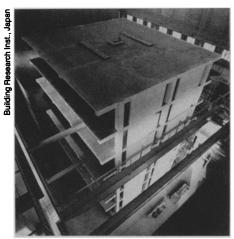
draulic jacks attached to a rigid adjacent wall. The tests took a week or two to simulate the inertial forces experienced in a 15-second quake.
