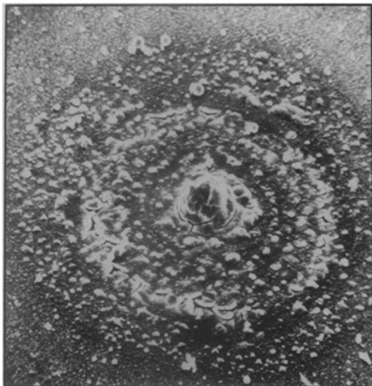
Shuttle exhaust droplet collected on copper plate reveals size in electron microphoto enlarged 425X.
