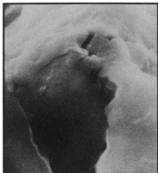
Quest for the core: The electron microscope's beam had to probe crevices like these within the droplet residue to find the aluminum oxide particle at the center, around which droplet condensed.
