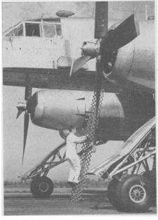
COLLAPSIBLE LADDER can be folded into a portable three-foot package easily carried by one man, although it is 15 feet long when expanded. Built on the principle of a collapsible gate, it is shown in the picture in use on the runway of the airplane company that developed it.
